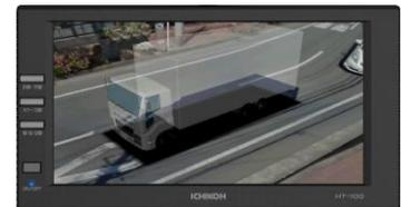
Even if drivers check using a normal back camera and side mirrors together, blind spots will occur behind the vehicle. This product technology makes it possible to check the side and rear of the vehicle on a single monitor, including spots that were difficult to be seen before.
