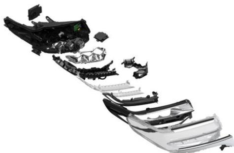
disassembled models of headlamp
