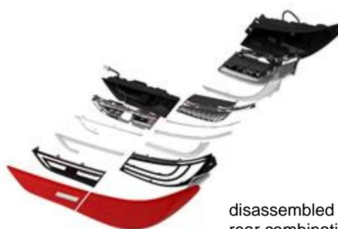
disassembled models of rear combination lamp
